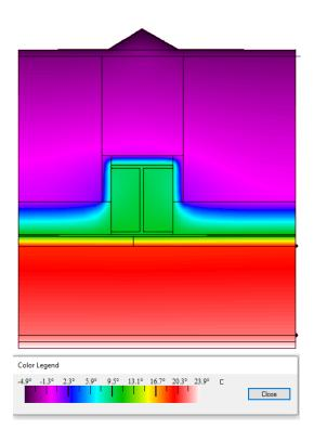
**Figure 5.** Covering "H" profiles with "Stone wool insulation 30 mm" to prevent sweating (Color infrared)
