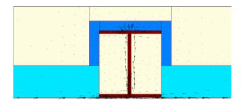
**Figure 6.** "Flux vector" indicator at the proposed insulation locations in the "H" profile sections
