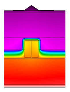
Figure 7. Thermal analysis of one layer of 100 mm stone wool (specific gravity 90 kg/m<sup>3</sup>)
